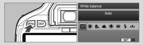
Press WB button, select the customer white balance on the display and confirm with the "set" button.
